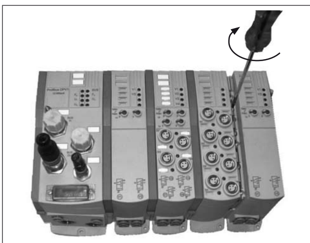
Fig. 9: Securing added modules
